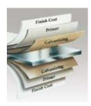
Steel skins are protected through a tough, layered coating system, including a hot-dipped galvanized layer, a protective metal oxide pretreatment and a bakedon primer and top coat.
